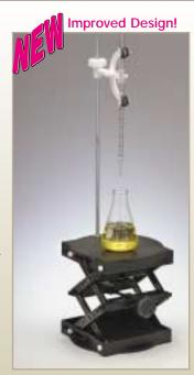
NOTE: The lab jack is not intended to be used to lift weight from its bottom position. Place the weight on the top plate only after raising to the desired height.
